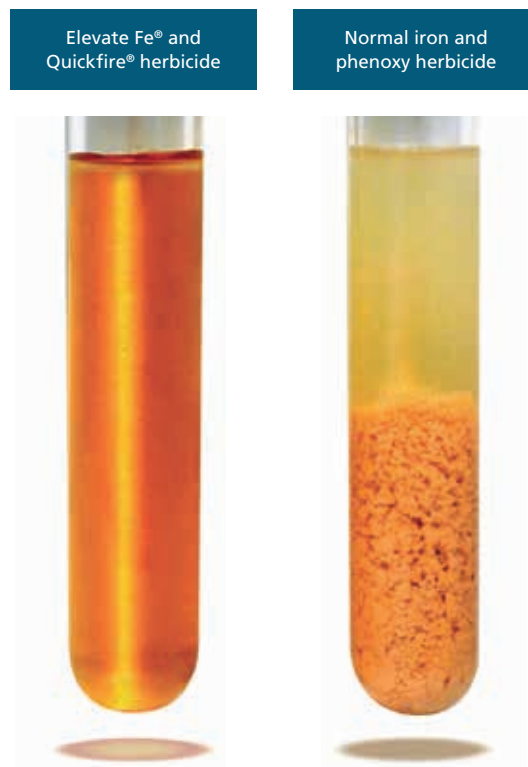
Fig. 1. Results of reactivity when Elevate Fe is used as a tank-mix component with Quickfire herbicide compared to normal iron and phenoxy herbicide.
